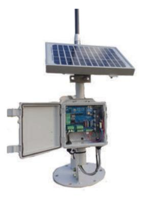
This system is a four channel radio telemetry unit, suitable for monitoring and or control applications, where no more than four inputs or outputs are required at the location.
